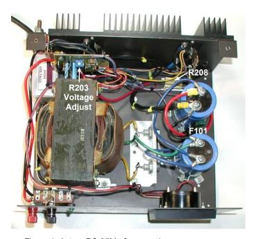
Figure 1. Astron RS-35M after rework.
