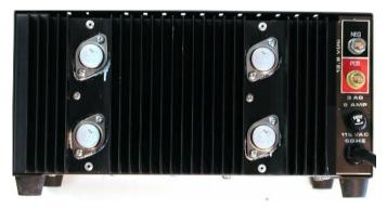
Figure 2. Astron RS-35M rear panel with new pass transistors.
