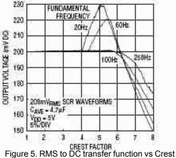
Figure 5. RMS to DC transfer function vs Crest Factor above 4:1. *Graph from LTC data sheet sn1966*
