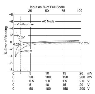
Figure 10. AC calibration and Linearity results for each range of the engineering prototype.
