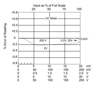
Figure 11. DC calibration and Linearity results for each range of the engineering prototype.
