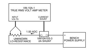
Figure 3. Lo-Ohm measurement using an external bench power supply with the VM-10A-1.
