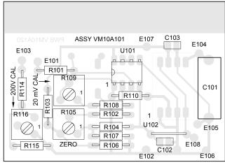
Figure 13. VM10A101 Assembly Component Locator.
