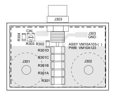
Figure 15. VM10A103 Assembly Component Locator.
