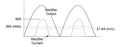
Figure 2. Peak, RMS and Average values of a current pulse typical of a shunt capacitor rectifier circuit.
