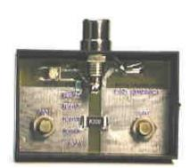
Figure 8. VM103A-2, 0.2 Amp Shunt typical of shunts -1, -2, -3. The -4 and -5 have additional copper sheet and 30 A posts.
