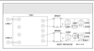
Figure 14. VM10A102 Assembly Component Locator.
