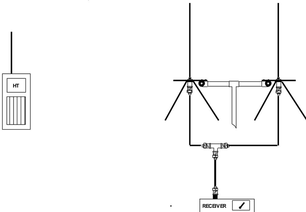
In an open area, use a HT to transmit a low power signal. Rotate the antenna and monitor the receivers meter to determine the exact location of null.
