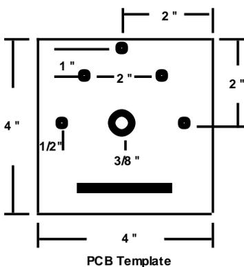
The screw and radial mounting holes are 1/8 "and the antenna connector is 3/8 ".
