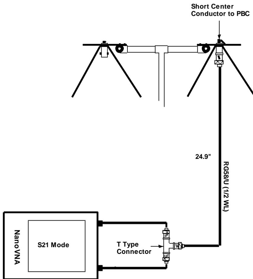
**1/2 Wavelength Measurement Setup**
