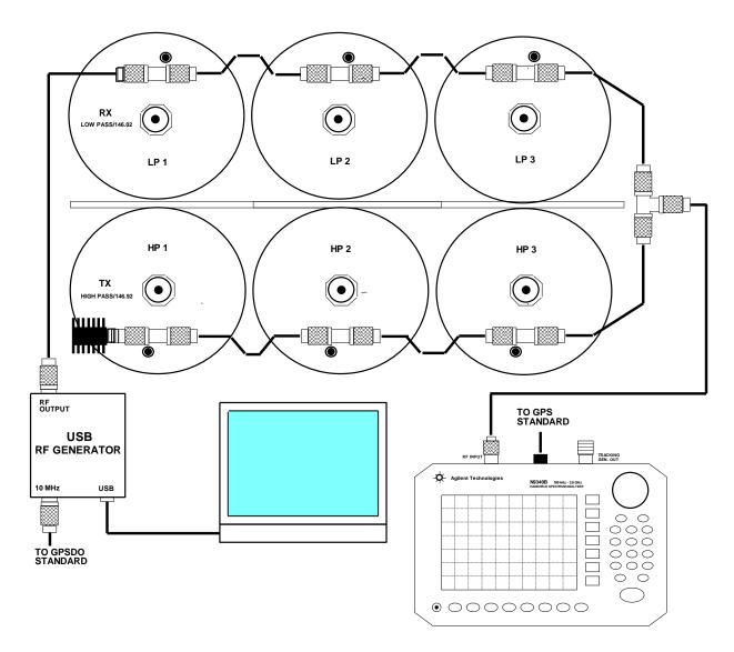
The suppression levels of 125 dB and 123 dB is well below the manufacturers 100 dB specification
