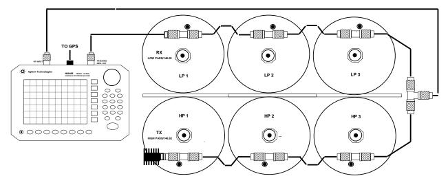
TX cavity sweep test setup
