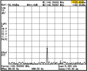
This measurement method allows you to determine if the noise suppression and receiver isolation meet the manufacturers specification. As a last resort, you can replace the spectrum analyzer with a 2M receiver, open its squelch and listen for a null. This will not allow you to determine if the rejection level meets the manufactures specifications.
