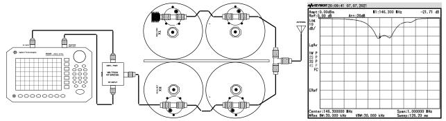
The screen plot below shows the results of adding 12.5 inches to the antenna feedline, the duplexers tuning was restored and the Return Loss was 38.14 dB. Note: Page 9 of this documents explains how the impedance of a coaxial cable can change when not terminated with 50 ohms. In this case, this phenomena was used to correct the impedance mismatch.
