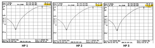
I've highlighted the High Pass insertion loss of this cavities. All of the TX cavities had similar insertion loss readings. According to the manufactures specifications, the maximum duplexer insertion loss is 2.2 dB. The total insertion loss for the 3 cavities was **3.91** dB which would result in low TX output power. The noise suppression was 33 to 36 dB which is in the normal range for a single cavity.
