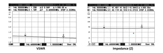
**Receiver Port Impedance Test:** The duplexer's antenna port was terminated with a 50 ohm load and a Return Loss Bridge was used to measure the RX port value. This test showed RX port Return Loss as being 40.2 dB with 50 ohm load which equals to a VSWR of 1.02:1. and an impedance of 51 ohms.
