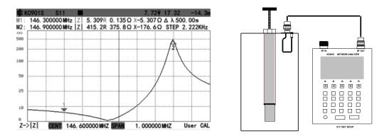
This VNA S11 Measurement of cavity port shows the impedance values from the pass and reject frequencies. Note: Normalize the VNA cable before taking this measurement.
