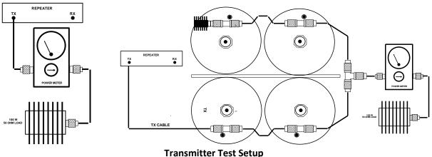
**Never** turn the band-pass tuning knob when attempting to correct an output power problem. Test the transmitter's output power by measuring the power when connected directly to a 50 ohm load. If you don't know the TX cavity insertion loss, it will need to be measured. The typical insertion loss for a 4 cavity duplexer is 1.6 dB and 2.2 dB for a 6 cavity unit.
