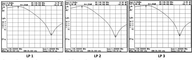
The total insertion loss is 1.85 dB and the total receive transmitter isolation 108.52 dB.
