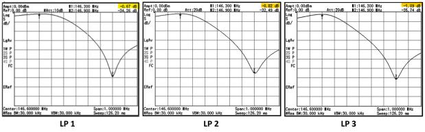
I've highlighted the Low Pass insertion loss which equaled to 1.9 dB. The RX insertion values were within the manufactures specifications. The TX cavities have a major problem, but RX duplexer cavities tested ok. Since the duplexer has been in service for over 20 years (8/2000), all of the cavities will need to be refurbished.
