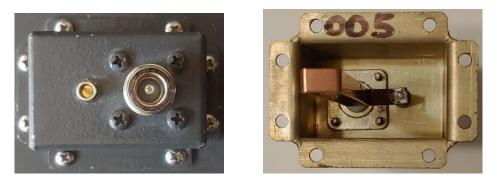
The 005 number on the assembly flange indicates that this coupling loop goes in a High Pass cavity. Coupling loops with 004 numbers go in the Low Pass cavities. If the coupling loop assembly flange does not have any number markings or if you need to verify that the marking is correct, you can compare the loop dimensions as seen below.
