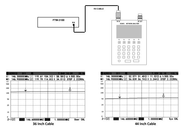
Connecting the Yaesu transceiver to the duplexer RX port with a 36" cable would destroy the RX cavity tuning and result in weak signal receiving problems. The 44" cable would provide 52.5 ohm match to the RX port at the 146.30 MHz RX frequency.
