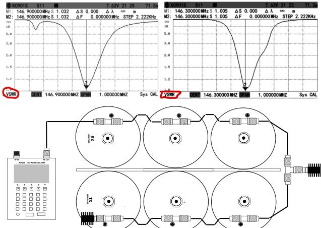
If the duplexers were properly designed, VSWR will usually provide the best RX and TX insertion Loss. Use the next test to measure the insertion loss to verify this is true. If you change any of the resonator settings, check the VSWR again to make sure it's within the manufacturer's 1.5:1 spec.
