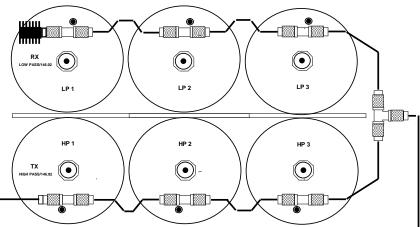
TX cavity sweep test setup
