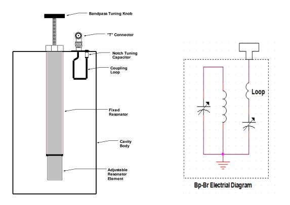
How the cavity Tee connector port reacts to impedance holds the secret of how Bp-Br cavities work. In this case, the cavity pass frequency was adjusted to 146.90 MHz and the reject frequency to 146.30 MHz.
