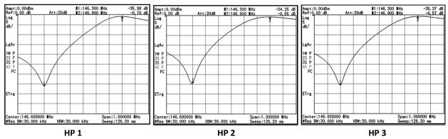
The total insertion loss is now 1.83 dB, compared to the 3.91 dB measured before cleaning the resonator adjustable element. Total transmitter noise suppression was 105.8 dB and this value will increase to a higher level when the  $\frac{1}{4} \lambda$  cables are installed.
