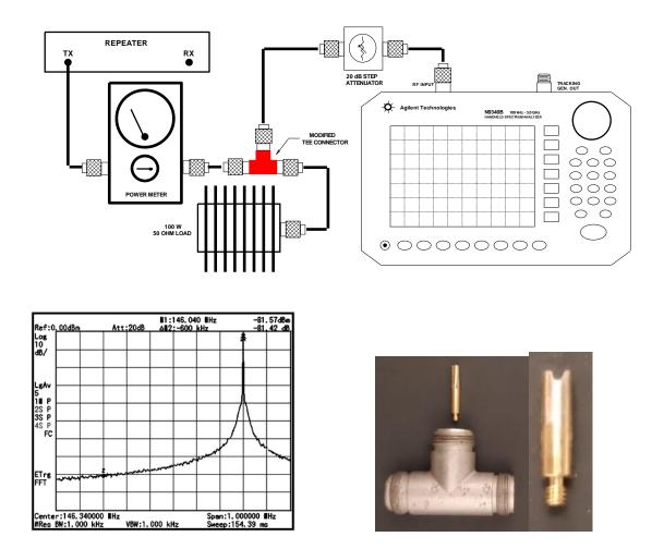
This test allows you to use a standard 50  $\Omega$  load, but requires you to modify a Tee connector so the spectrum analyzer is not destroyed. Tee Connector Modification: Remove the connector center pin and break off the fingers and replace the center pin. The connector modification provides 40 to 50 dB of attenuation across a frequency of 144 – 148 MHz.
