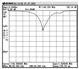
Receive port Return Loss with the antenna feedline length increased by 12.5 inches.
