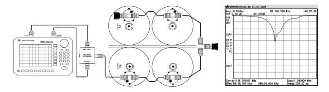
Replacing the 50 ohm load with the antenna not only caused a change in Return Loss response, it reduced the Return Loss value to 21.7 dB.
