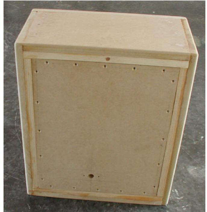
**Figure 2.** Speaker box viewed from back. Double cleats are used for the back to reduce the slab area and stiffen the side to back corners.
