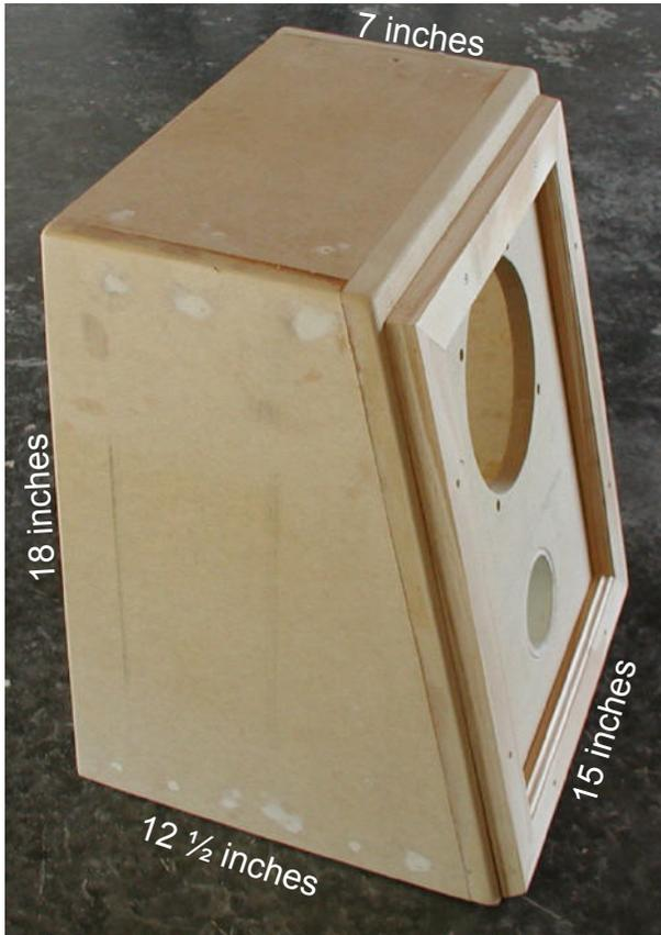
**Figure 1.** Speaker box viewed from front and side. The speaker frame is attached for fitting and the port is visible below the driver opening. Note the dimensions are inside dimensions required to meet the 1.56 cubic foot volume.
