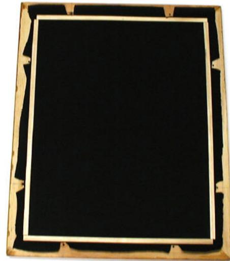
**Figure 4.** Speaker grill cloth frame from the back side. The grill cloth is stretched and clamped into 3/8" dado cut 5/16" deep into the frame. Wooden strips are cut and planed to wedge fit the cloth into the dado. Note grill cloth is cut away from the screw holes to void being pulled by the screws upon installation.
