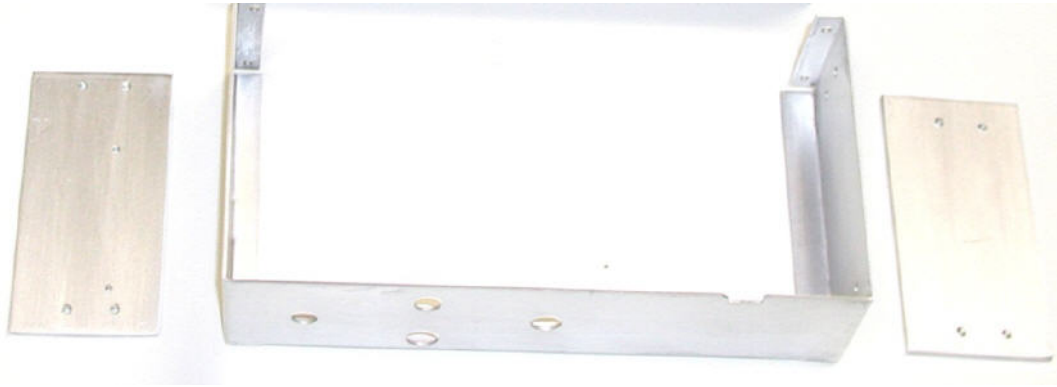
Figure 4. Internal chassis serves to mount the front and back panels, support the circuit board and provide attachment of the clam shell covers by supporting the threaded 0.125" aluminum plates.
