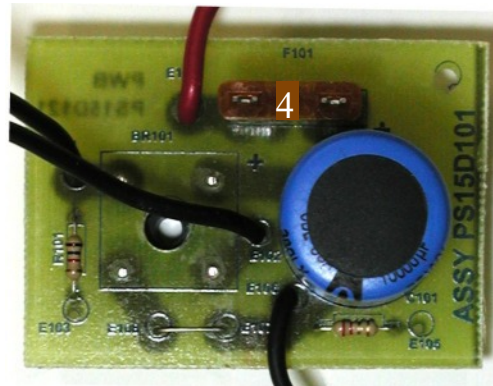
Figure 15. PS15D101 Rectifier Assembly. Note BR101 is mounted on foil side of PWB for heat sink attachment.
