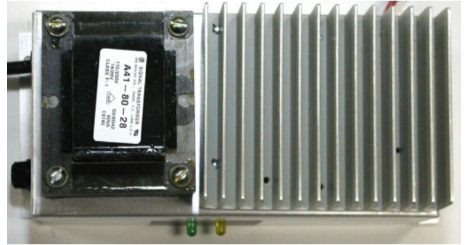
Figure 20. PS-15D-1 top view . Heat sink mounts on chassis which has a cut-out for Q1 to mount directly on the heat sink.
