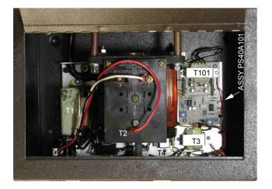
Figure 1. Top view, looking down into steel enclosure. Front panel is at the bottom and the variac, T2, is in the center and assembly PS40A101 is to the right.
