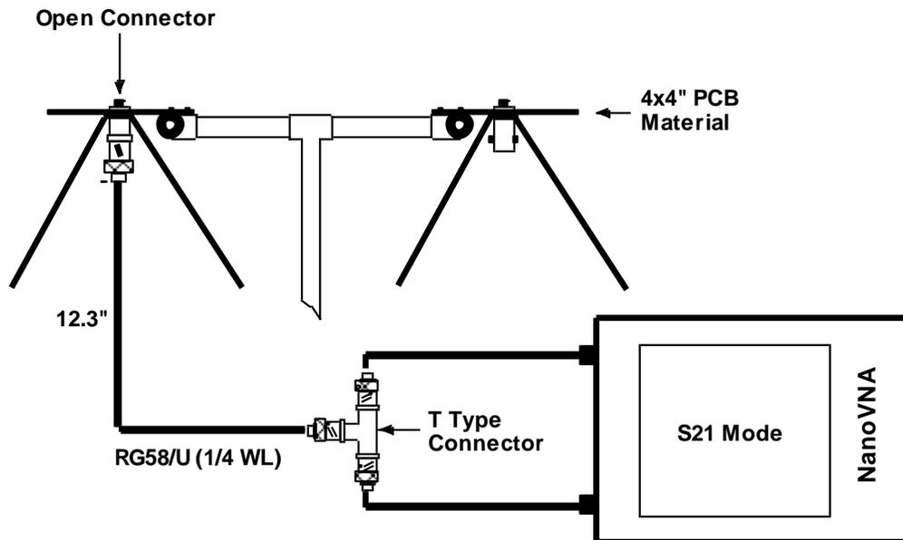
1/4 Wavelength Test Setup
