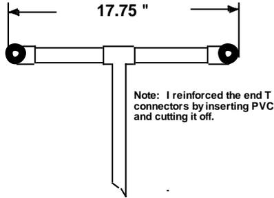
Install the BNC connectors on the PCB antenna mounting plates. Place the mounting over the T connector and mark the back center hole, the drill a 3/32 pilot and the plate with a self-tapping screw. Then drill the pilot holes for other two mountings. Caution: Make sure the antenna connector center pins are separated by 19.25".
