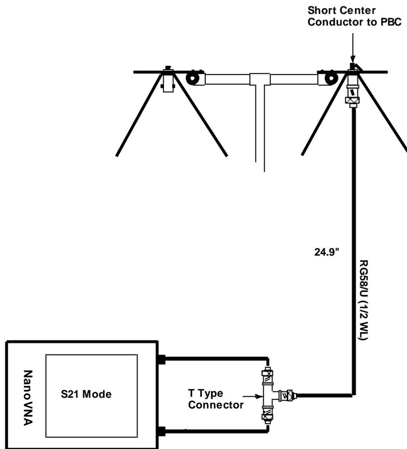
**1/2 Wavelength Measurement Setup**
