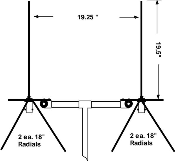
With the driven elements installed, it's time to adjust the 1/4 wavelength antennas for the best SWR at the 146.00 MHz frequency.
