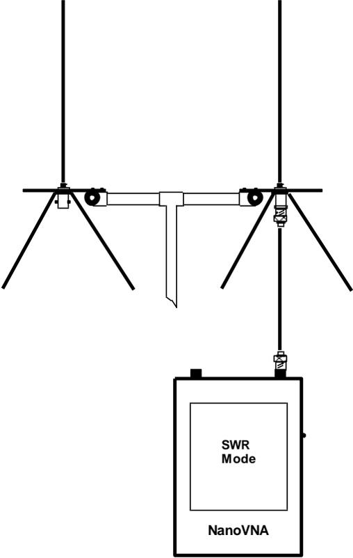
Use this test setup to adjust both antennas, theirs's a minimal of interaction between the antennas. Make sure you normalize the cable used between the VNA.
