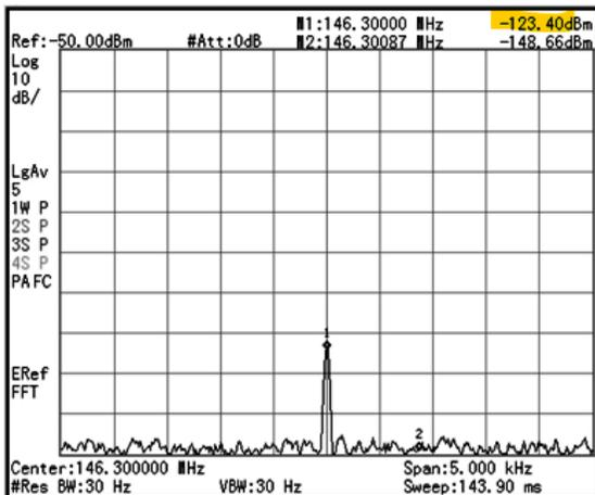
The RF generator output is adjusted for 0 dBm so the notch level can be read directly. Since this noise suppression level determines the sensitivity of the repeaters receiver, it's important that the generators be accurate.
