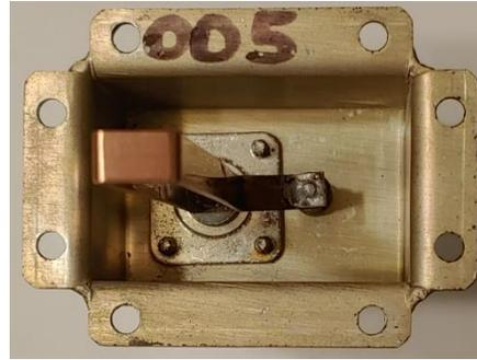
The 005 number on the assembly flange indicates that this coupling loop goes in a High Pass cavity. Coupling loops with 004 numbers go in the Low Pass cavities. If the coupling loop assembly flange does not have any number markings or if you need to verify that the marking is correct, you can compare the loop dimensions as seen below.
