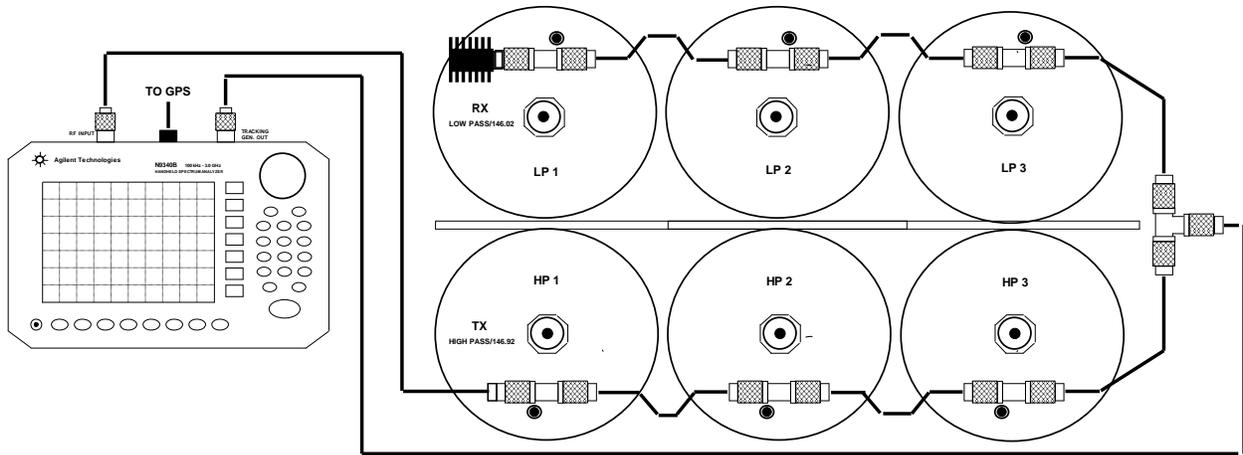
TX cavity sweep test setup
