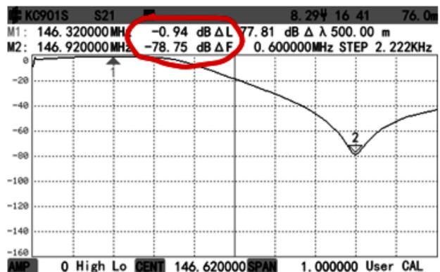
**Both Cavities connected with a 10.5 inch Cable**
