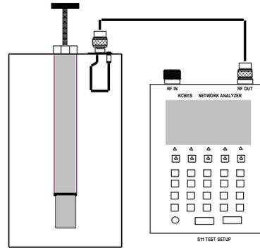
This VNA S11 Measurement of cavity port shows the impedance values from the pass and reject frequencies. Note: Normalize the VNA cable before taking this measurement.
