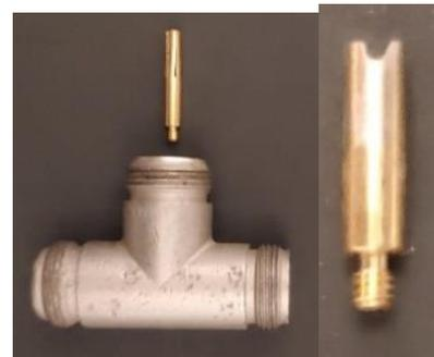
This test allows you to use a standard 50 Ω load, but requires you to modify a Tee connector so the spectrum analyzer is not destroyed. Tee Connector Modification: Remove the connector center pin and break off the fingers and replace the center pin. The connector modification provides 40 to 50 dB of attenuation across a frequency of 144 – 148 MHz.
