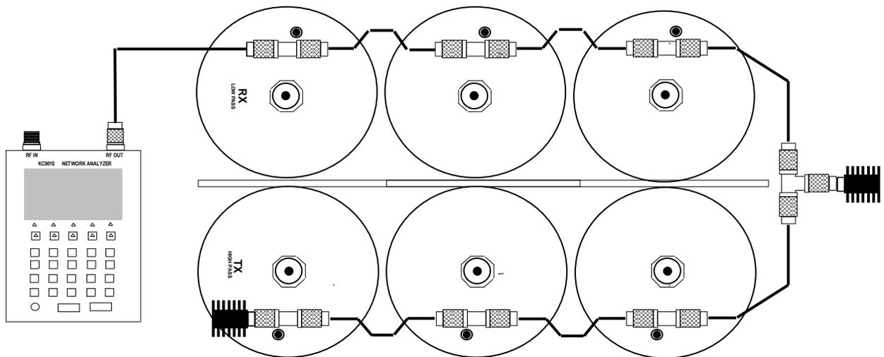
If the duplexers were properly designed, VSWR will usually provide the best RX and TX insertion Loss. Use the next test to measure the insertion loss to verify this is true. If you change any of the resonator settings, check the VSWR again to make sure it's within the manufacturer's 1.5:1 spec.
