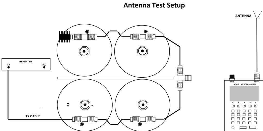
Looking at the antennas VSWR, the 146.30 MHz (RX) frequency reading was **1.258:1** which would be considered as good value if it was connected to your mobile radio. The impedance measurement shows that the impedance 41.0 and 42.1 ohms, which not be a impedance match for the duplexers antenna port.
