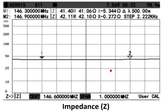
**Receiver Port Impedance Test:** The duplexer’s antenna port was terminated with a 50 ohm load and a Return Loss Bridge was used to measure the RX port value. This test showed RX port Return Loss as being 40.2 dB with 50 ohm load which equals to a VSWR of 1.02:1. and an impedance of 51 ohms.
