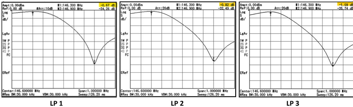
I’ve highlighted the Low Pass insertion loss which equaled to 1.9 dB. The RX insertion values were within the manufactures specifications. The TX cavities have a major problem, but RX duplexer cavities tested ok. Since the duplexer has been in service for over 20 years (8/2000), all of the cavities will need to be refurbished.
