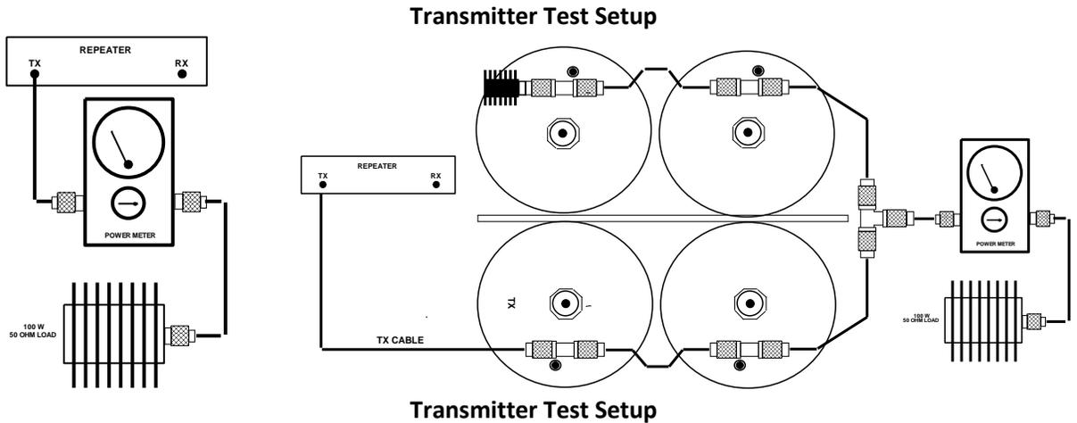
**Never** turn the band-pass tuning knob when attempting to correct an output power problem. Test the transmitter's output power by measuring the power when connected directly to a 50 ohm load. If you don't know the TX cavity insertion loss, it will need to be measured. The typical insertion loss for a 4 cavity duplexer is 1.6 dB and 2.2 dB for a 6 cavity unit.
