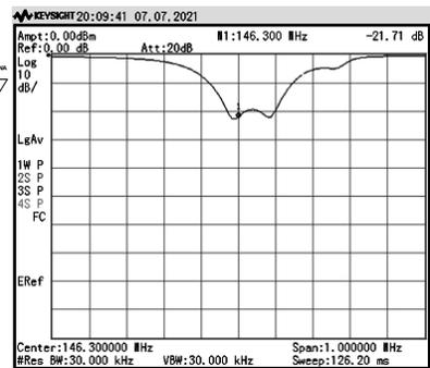
The screen plot below shows the results of adding 12.5 inches to the antenna feedline, the duplexers tuning was restored and the Return Loss was 38.14 dB. Note: Page 9 of this documents explains how the impedance of a coaxial cable can change when not terminated with 50 ohms. In this case, this phenomena was used to correct the impedance mismatch.
