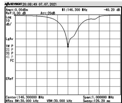
Replacing the 50 ohm load with the antenna not only caused a change in Return Loss response, it reduced the Return Loss value to 21.7 dB.
