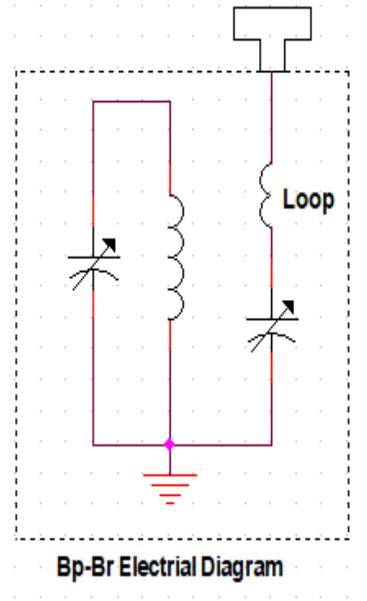
How the cavity Tee connector port reacts to impedance holds the secret of how Bp-Br cavities work. In this case, the cavity pass frequency was adjusted to 146.90 MHz and the reject frequency to 146.30 MHz.
