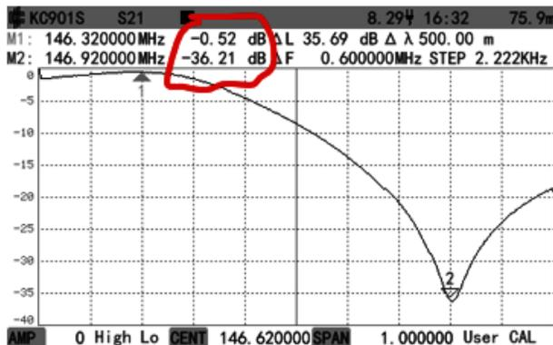
**Each Cavity Rejection -36.2 dB @ 146.92 MHz**
