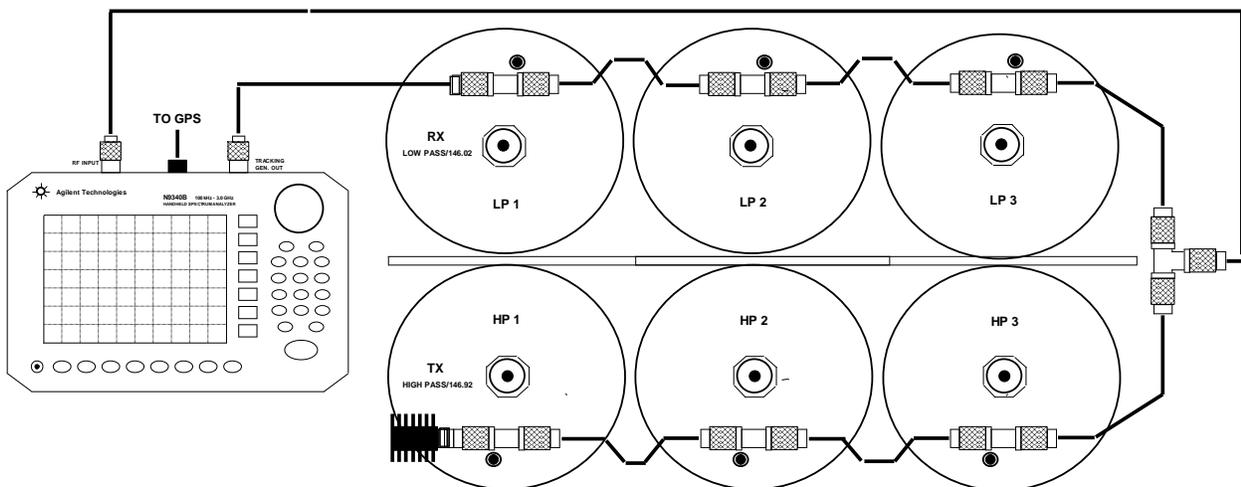
TX cavity sweep test setup
