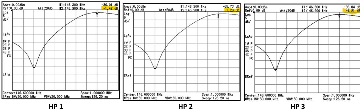
I've highlighted the High Pass insertion loss of this cavities. All of the TX cavities had similar insertion loss readings. According to the manufactures specifications, the maximum duplexer insertion loss is 2.2 dB. The total insertion loss for the 3 cavities was **3.91 dB** which would result in low TX output power. The noise suppression was 33 to 36 dB which is in the normal range for a single cavity.
