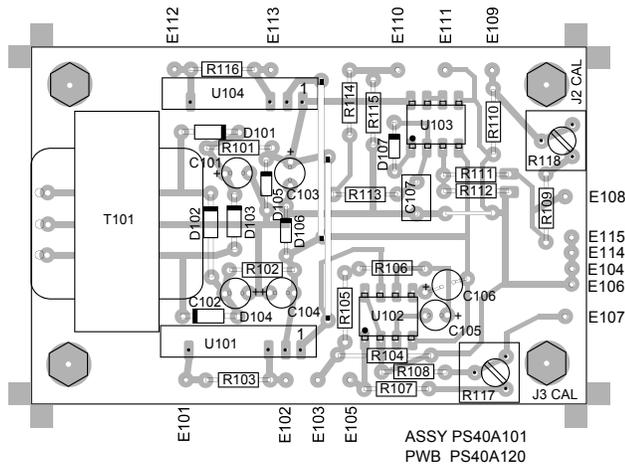
Figure 3. Component locator for assembly PS40A101.
