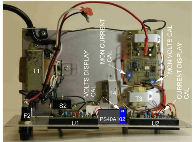
Figure 2. Top view of chassis - removed from the steel enclosure. Note locations of key components and calibration points.
